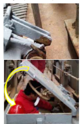
Hook slipped off, hatch fell and hit the head hardly
